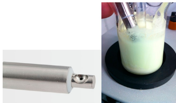
Figure 7. Autosampler that is introduced in the reaction vessel.
