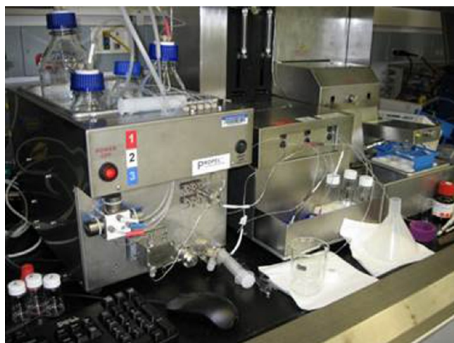
Figure 21. Laboratory-based screening tool for flow chemistry evaluation.
